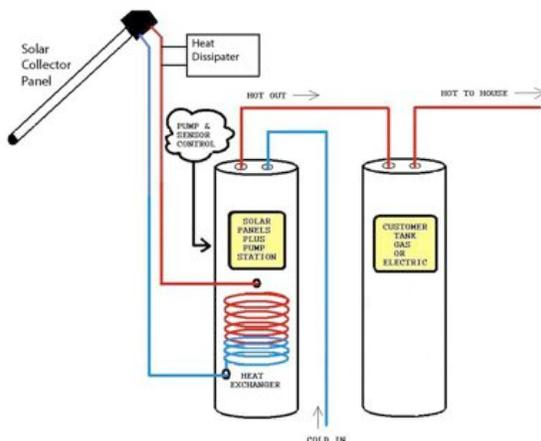
The panels for a closed loop system (shown above) are comprised of glass tubes with a copper heat transfer mechanism. See [Solar Panels Plus: How Solar Hot Water Heaters Work](#) for a great description; their diagram is shown, left (10).
