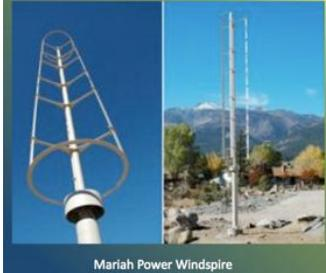
Wind is all about location, and for most of the Flathead Valley, it's not good. Also, the turbine should be about 30 feet above the surroundings to work.
